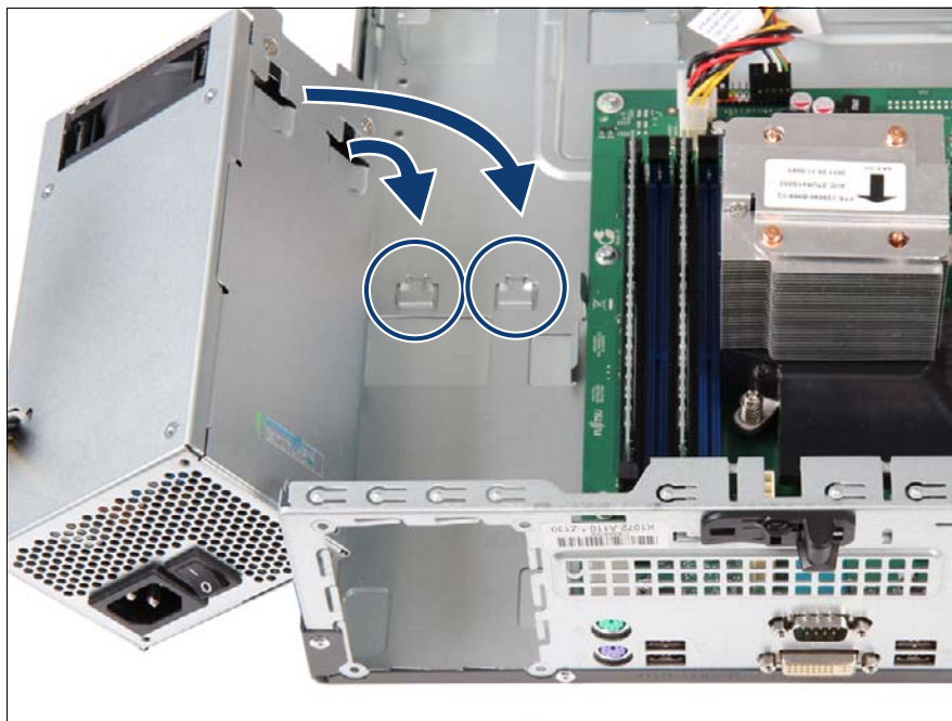
Figure 18: Installing the standard PSU
